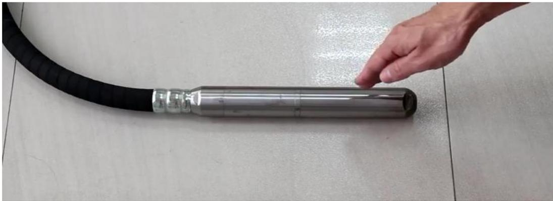
It uses a high frequency motor mounted directly in the vibrator head with generates 12500VPM for fast and effective removal of air bubbles. The vibrator head has a hardened steel casing and heavy duty bearings.
