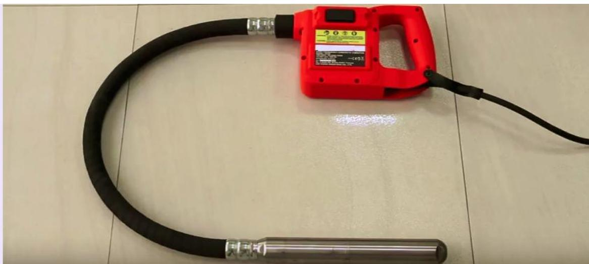
High frequency has many advantages over flex-cable systems powered by universal motors. The high frequency motor design maintains consistent speed, losing less than 5% of its no-load VPM. Even in heavy, low slump concrete – A flex shaft vibrator can lose 40% or more of its VPM under heavy load.
