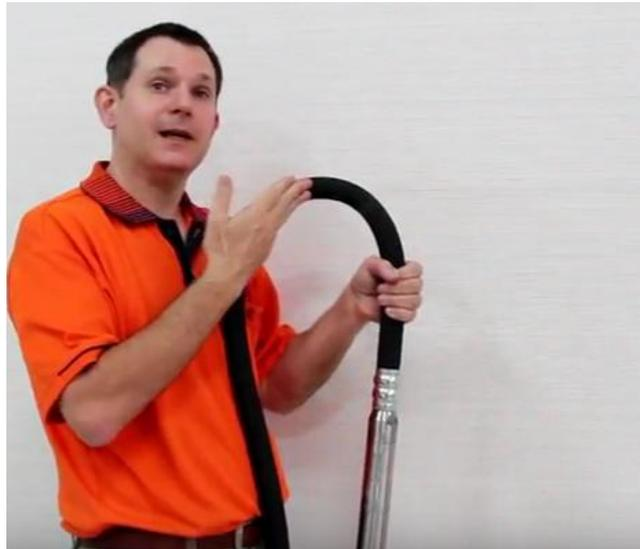
Since the hose only contains electric wires, there is no flexible drive shaft. So there are no friction losses and no need to worry about over-bending the hose (as you would with a flex-shaft driven design)
