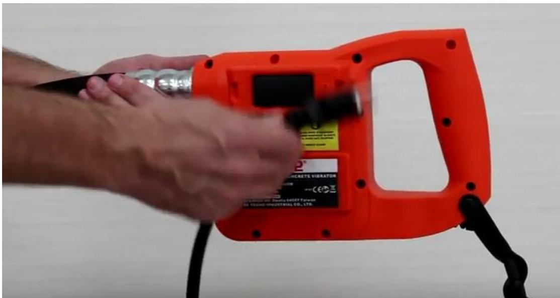
It contrasts to traditional high frequency systems, which require a separate frequency converter. This machine has the converter integrated into the handle, so one can simply plug into the standard single phase current available on any jobsite. This makes operation much simpler and more convenient, giving the operator of each unit total autonomy of movement.
