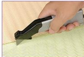
Standard blade for cutting cardboard or plywood
