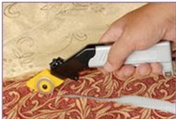
Circular blade for cutting textile materials and leather
